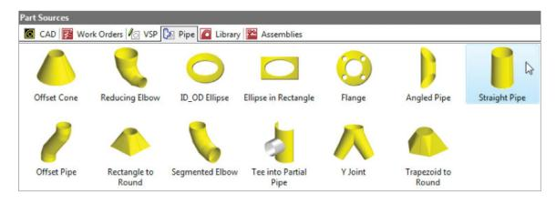
Customizing developments in ProNest is simple. You'll be able to set dimensions and add various shape tee branches, including conical, cylindrical, rectangular, or boot format. Each fitting can be adjusted to your needs with powerful features like offsets, tilts, extensions, and laps.
